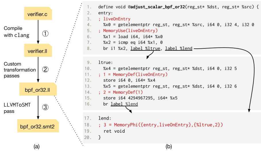
Fig. 4: (a) The pipeline for automatically generating an SMT-LIB file from the Linux kernel’s verifier.c . Shown here is an instance of the pipeline for the bpf_or32 instruction. (b) The LLVM IR presented as a CFG, overlaid with MemorySSA analysis in red, for a function adjust_scalar_bpf_or32 that is representative of verifier code for bpf_or32 . It takes as input two structs dst and src and modifies them.
